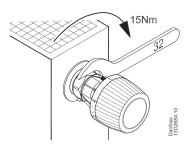
Built-in sensors should always be fitted horizontally so that the ambient air can pass freely over the sensor.
